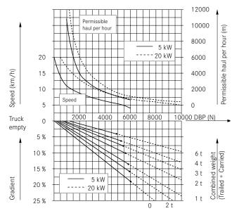
The permissible haul per hour is the total distance travelled, including the return journey and any downhill gradients.
